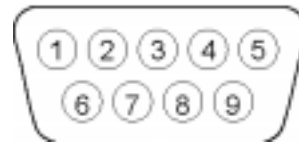
RS-232 Connector Pin Layout.
