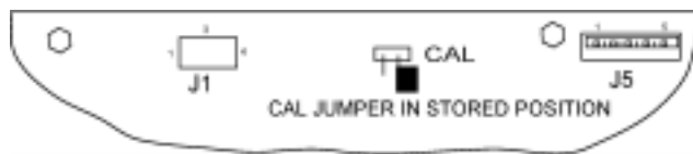
CAL Jumper Shown in Stored or ON Position.
