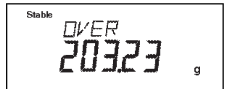
OVER is displayed for weights greater than or equal to the OVR WT limit
